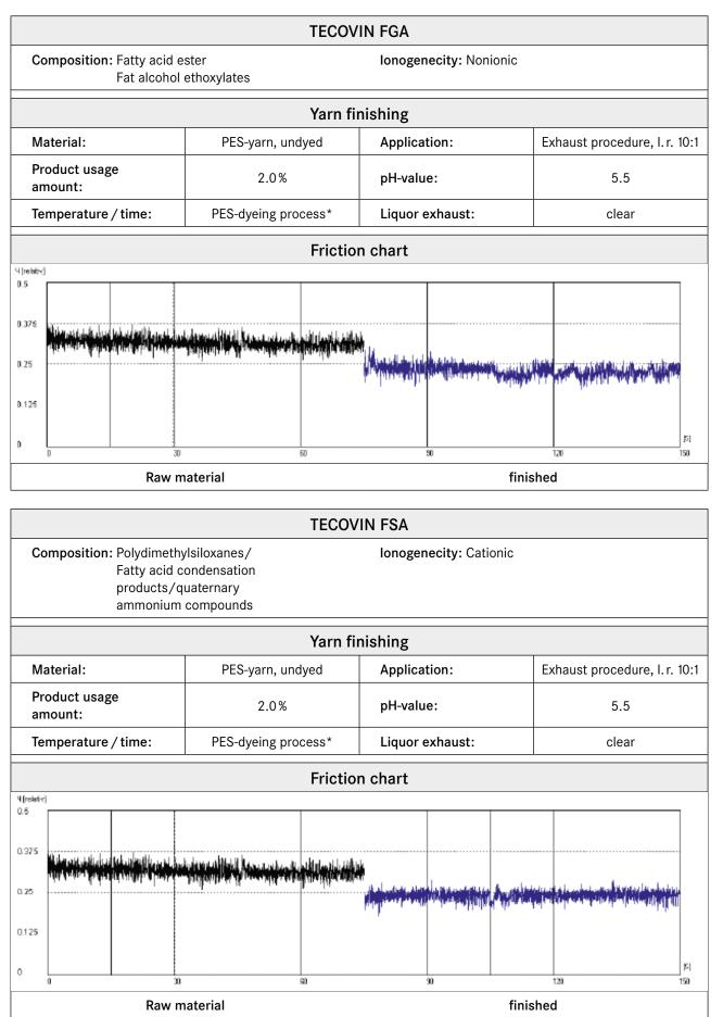
\*Bind dyeing: 130 °C/45 min, cool down to 80 °C, reductive clearing: 0,5 g/l Tecoredukt 1000 + 1.0 g/l Tc-Dispergator BL + 4.0 ml/l NaOH 38 °Bé 80 °C/20 min
