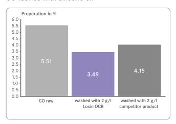
PA knitwear and CO fabric were padded with 50 g/l silicone oil AK-5000 and dried at room temperatures. The application volumes of PES/WO-fabrics were determined before and after conventional washing.
