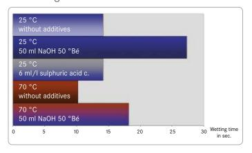
The good wetting effect of **Losin OCB** at room temperature is not impaired by strong acids. High alkali additions slow wetting. Higher temperatures increase the wetting effect.
